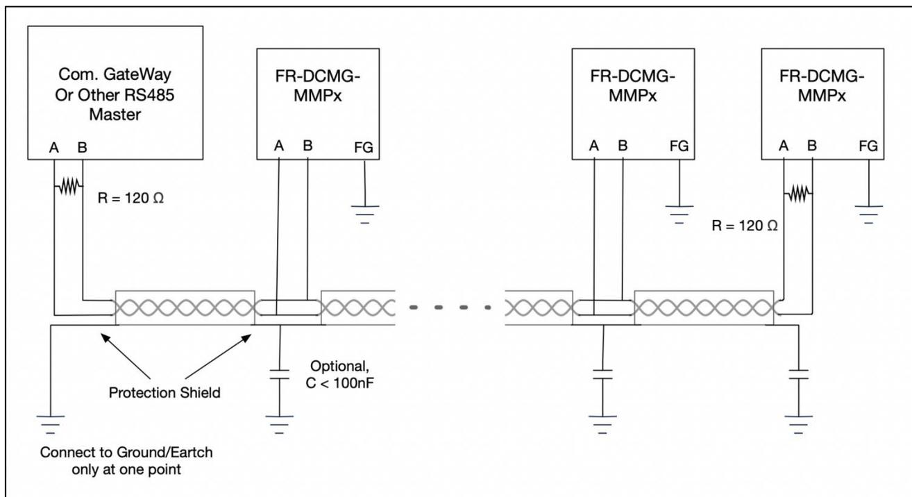
The wiring specifications of the communication shielded wire are shown in the figure above: The wiring of on-site communication lines requires that the communication shield can only be grounded at a single point, otherwise there will be a risk of lightning surge damage to all equipment on the entire communication line during a lightning strike;
