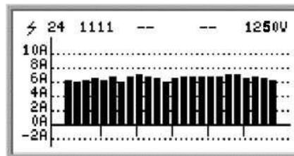
The histogram in the figure shows the current value detected by each channel. The initial interface display range is: -2A ~ 10A. You can also set register 0x0B16, which displays -2A ~ 20A and -2A ~ 30A. Because a six-channel Hall sensor is connected, every
