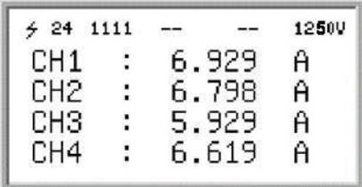
The value of cumulative power generation. When viewing the values of current and cumulative power generation, you can scroll through the screen by continuing to press the "+" or "-" key. After the current display is completed, continue to press the "+" key to start displaying the cumulative power generation. The figure above shows the current display interface. "CH1:" in the figure indicates that the current value monitored by channel 1 in real time is "6.929A" , and so on.
